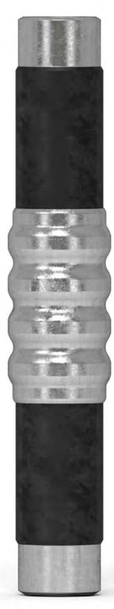
Mechanical electroinsulating connection of pipelines (MEST<sup>M</sup>) is designed for electrical isolation of pipelines from other underground structures. The purpose of electrical isolation is elimination or limitation of stray currents in the pipeline inducing by earth connections of direct or periodic currents in a high-voltage power transmission line and suppression of protective currents scattering of electrochemical (especially ground) corrosion protection.
