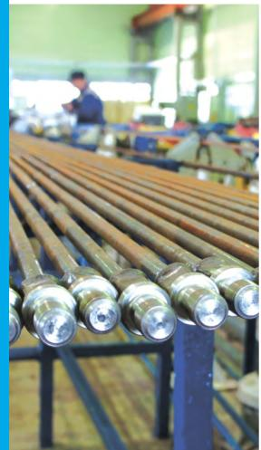
Pump rods of TMC group are produced on modern imported and home equipment made of highquality alloy steel with method of arc melting. At that chemical composition is chosen in such a way that physical and chemical properties of rod such as ductility, impact strength, fatique strength, wear and corrosion resistance are balanced for use in wells with abnormal geologic and technical conditions.
