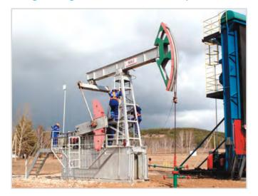
maintenance and repair of sucker-rod pump drives (beam pumping units and chain drives);
