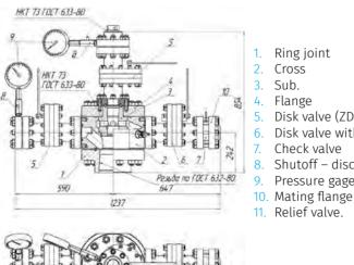
Ring joint Cross Sub. Flange Disk valve (ZD) Disk valve with choke valve (ZDSH) Check valve Shutoff – discharge unit (gage valve). Pressure gage Mating flange
